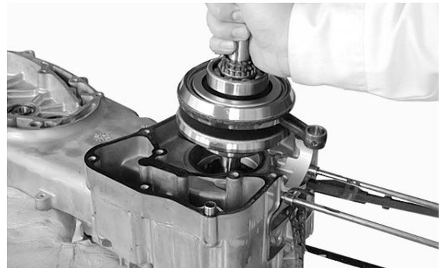
Clean off all gasket material from the crankcase mating surfaces.
