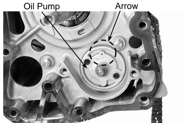
After the oil pump is installed, tighten the two mounting bolts.
