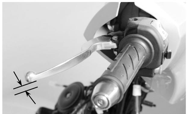
If the free play do not fall within the limit, adjust by turning the adjusting nut.
