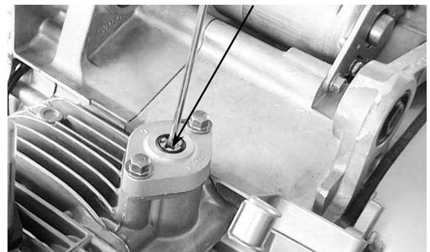
Turn the flywheel counterclockwise so that the "T" mark on the flywheel aligns with the index mark on the crankcase to bring the round hole on the camshaft gear facing up to the top dead center on the compression stroke.
