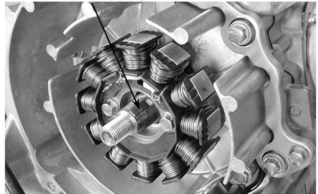
Install the flywheel onto the crankshaft with the flywheel hole aligned with the crankshaft woodruff key.
