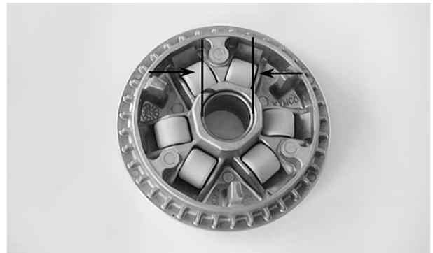
Check the drive pulley bushing for wear or damage.
