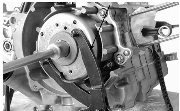
Hold the flywheel with the universal holder and tighten the flywheel nut.
