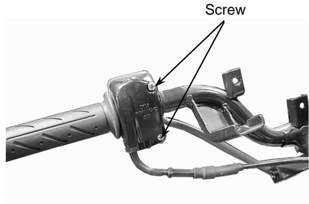
Remove the throttle seat from the handlebar and disconnect the throttle cable from the throttle pipe.
