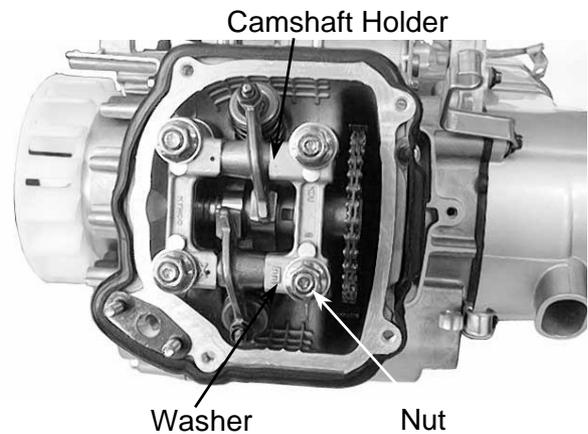
Adjust the valve clearance. (⇨3-5)
