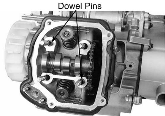
Install the camshaft holder, washers and nuts on the cylinder head.
