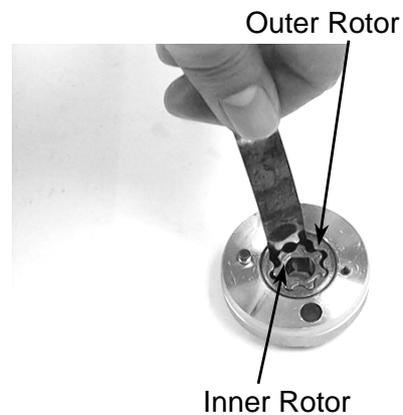
Measure the rotor end-to-pump body clearance.
