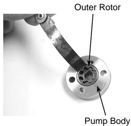
Measure the inner rotor-to-outer rotor clearance.
