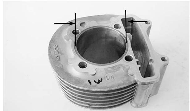
The true roundness is the difference between the values measured in X and Y directions.
