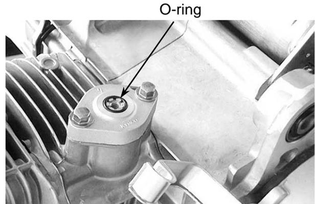
Install a new cylinder head cover gasket and
