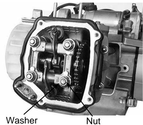
Remove the camshaft holder and dowel pins.
