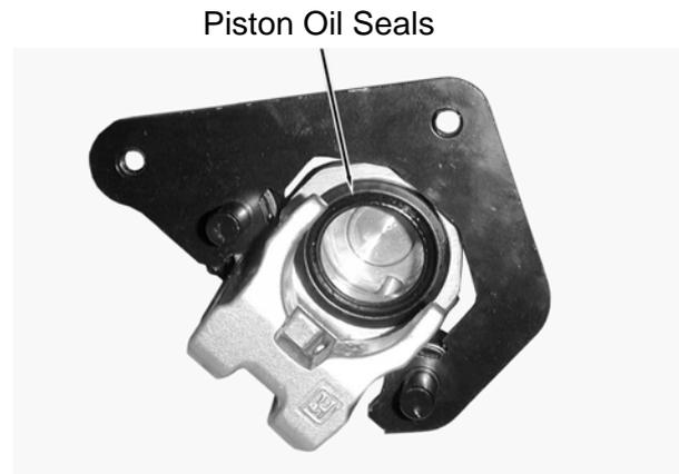
Check each piston for scratches or wear. Measure each piston O.D. with a micrometer gauge.
