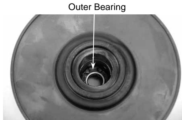
Seat the snap ring in its groove. Apply grease to the driven face bore areas.
