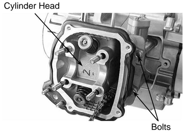
Remove the dowel pins and cylinder head gasket.
