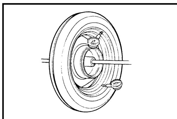
Turn the inner race of each bearing with your finger to see if they turn smoothly and quietly. Also check if the outer race fits tightly in the hub.
