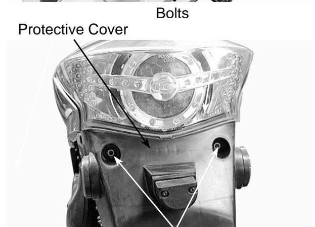
Remove the two screws on the bottom of the
