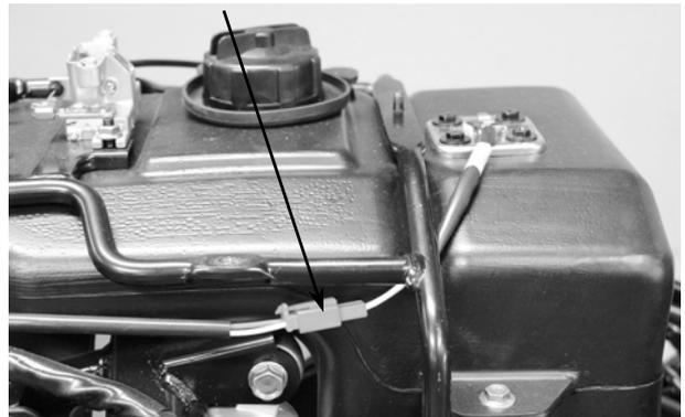
Disconnect the fuel tube and vacuum tube at the auto fuel valve.
