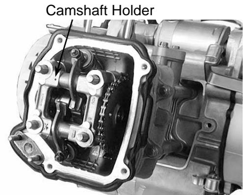
Remove the camshaft gear from the cam chain and remove the camshaft.
