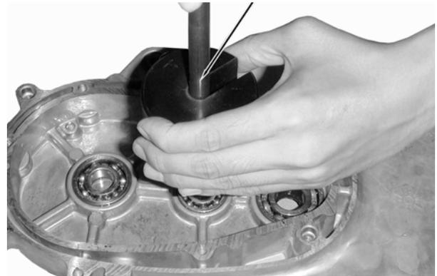
Drive new bearings into the left crankcase.
