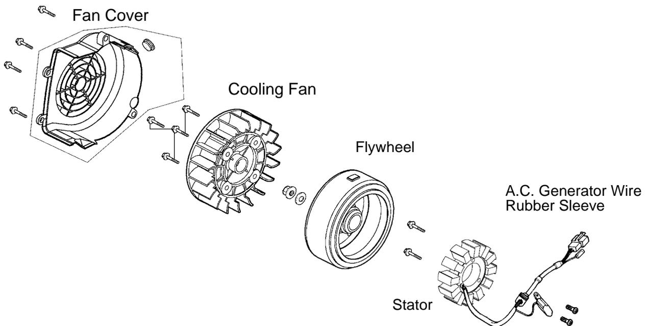
Install the A.C. generator stator and pulser coil onto the right crankcase.
