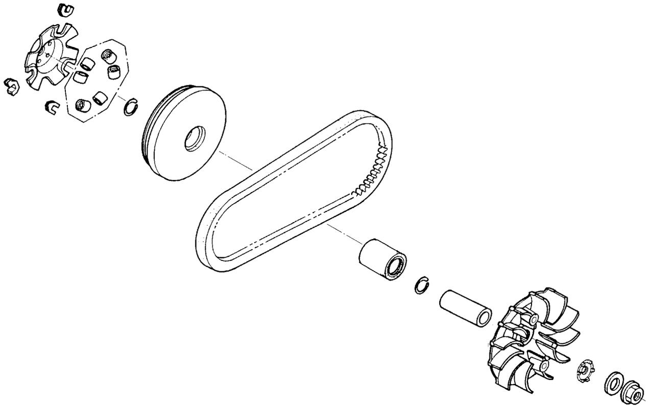
Install the weight rollers into the movable drive face.
