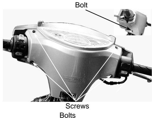
Remove the three nuts attaching the handlebar cover
