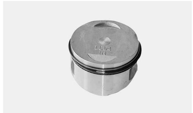
Install the piston rings onto the piston and measure the piston ring-to-groove clearance.
