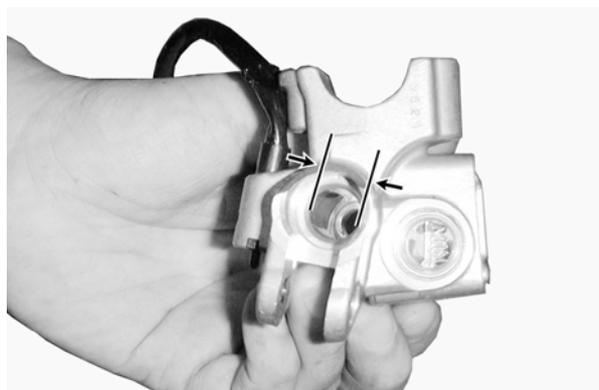
Measure the brake master cylinder piston O.D.
