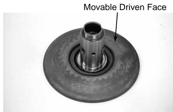
Install the movable driven face onto the driven face.
