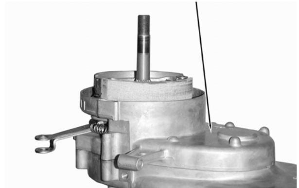
Install and tighten the transmission case cover bolts.
