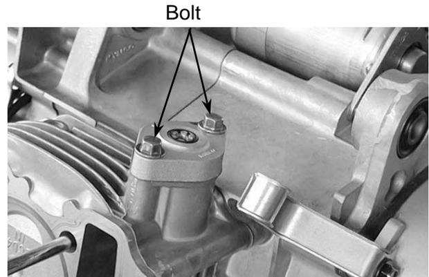
Remove the cylinder head. (⇒7-7)
