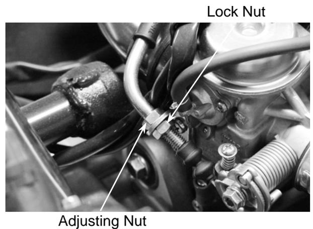
Minor adjustment is made with the adjusting nut at the throttle grip side.
