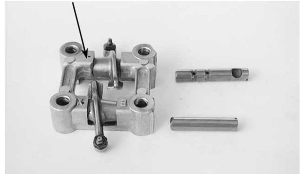
Measure the I.D. of each valve rocker arm.
