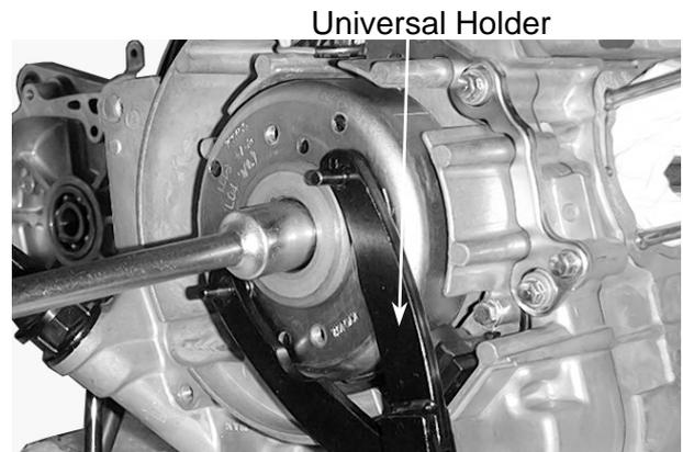
Remove the A.C. generator flywheel using the flywheel puller.
