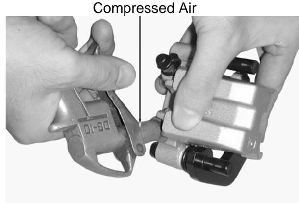
Push the piston oil seals outward to remove them. Clean each oil seal groove with brake fluid.
