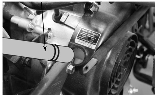
Also use a timing light to check the advance mark. Raise the engine speed to 5,000rpm and the index mark on the crankcase should be aligned with the advance mark on the flywheel.
