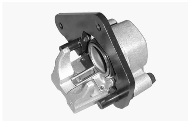
Wipe off excessive brake fluid with a clean shop towel. Apply silicon grease to the brake caliper seat pin and caliper inside. Install the brake caliper seat.
