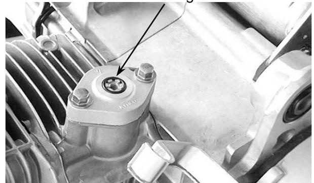
Turn the cam chain tensioner screw clockwise to tighten it.
