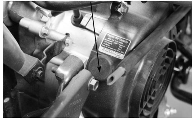
Check the ignition timing with a timing light. When the engine is running at idle speed, the ignition timing is correct if the "F" mark on the flywheel aligns with the index mark on the crankcase.
