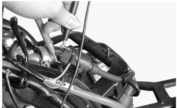
Measure the secondary coil resistances with and without the spark plug cap.
