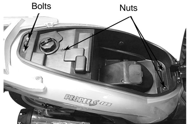
Remove the three bolts attaching the rear
