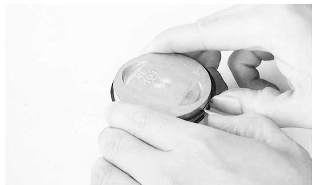
Remove the piston rings and insert each piston ring into the cylinder bottom.
